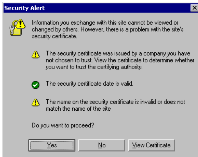
Figure 3-9 Security Alert Dialog Box for the Certificate (Displayed Statements and Icons may be Different)
