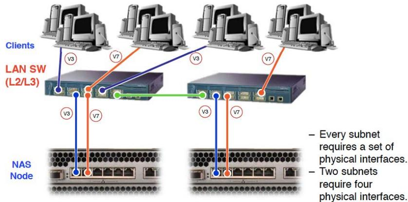
In this example, each separate subnet requires a minimum of one dedicated interface placed into a unique link aggregation group. Therefore, two subnets require four physical interfaces.
