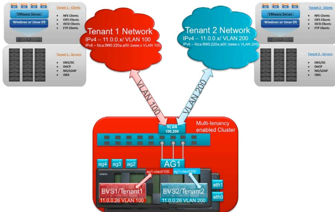
Incoming requests and outgoing responses are made with the EVS in context. The solution provides security between environments by performing crosschecks of server addressing, interfaces and virtual nodes as data is passed between stacks.
