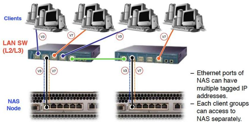
In this example, multiple tagged VLANs may share the same interfaces and link aggregation groups. It is also possible for both tagged and untagged (default) VLANs to be used simultaneously by the same switch ports.
