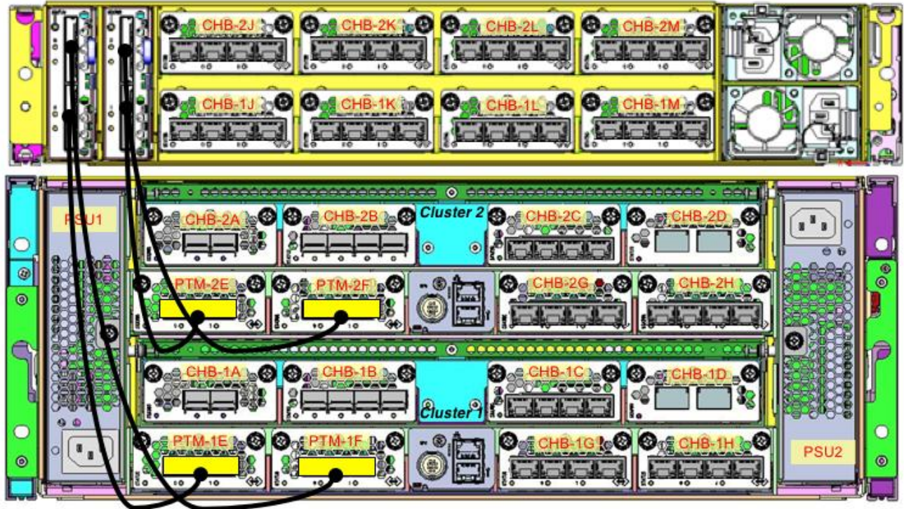
Figure 9: VSP G900 Controller Chassis (DKC) Organization with I/O Expansion Box -- Diskless
